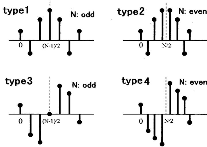
Figure 1: Four types of FIR filter
