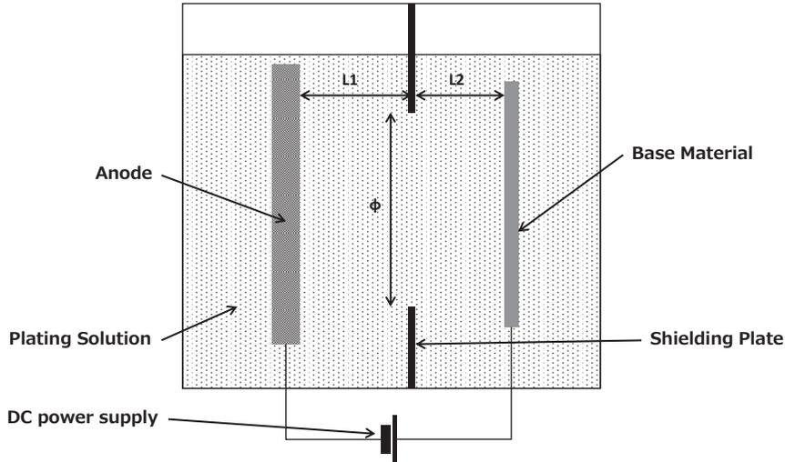
Figure 1 Principle of common electroplating process
